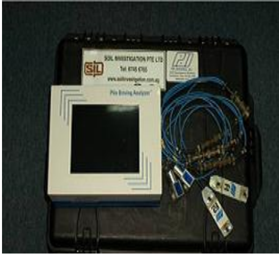
Figure 2.4 Pile Driving Analyzer
