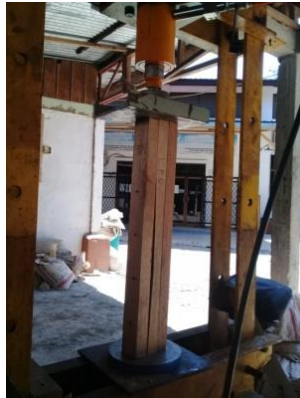
Figure 3 Compression Testing of Built-up columns
