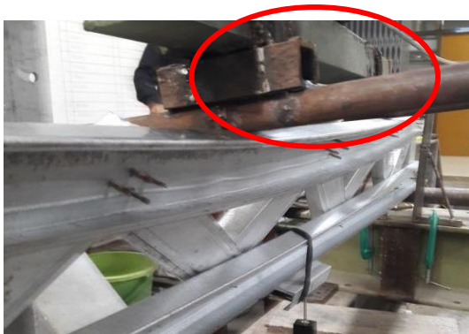
Picture 8. Failure of B-II Non Centric C Profile Beam
