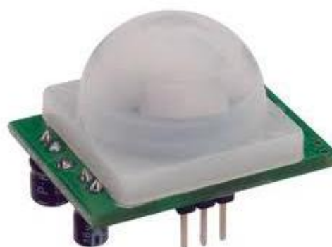
Figure 2.2. Sensor PIR (Passive Infra Red) (Ostadz, 2021)
