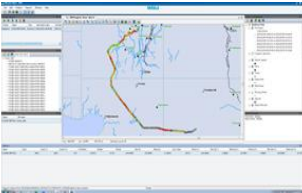
Figure 3. Lightning Density Map on the 500kV Depok-Tasik conductor in 2021
